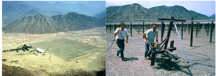
Fig. 1. The large array of the Jicamarca Radar (Left). Ken Bowles (with wheelbarrow) and then graduate student M.G.M. (Right), and a close-up view of the field of crossed dipoles. Images courtesy of the Bowles family.
