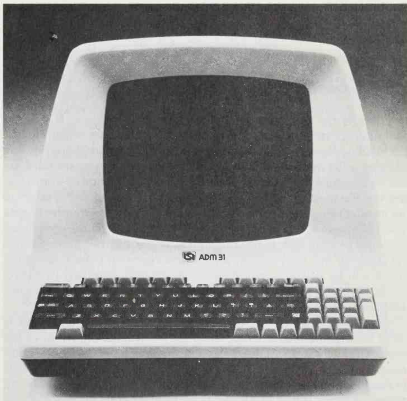
Figure 1.1: A CRT Terminal
