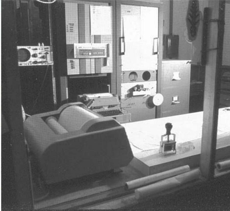
**Packard-Bell PB250 computer with mercury delay-line memory.**
