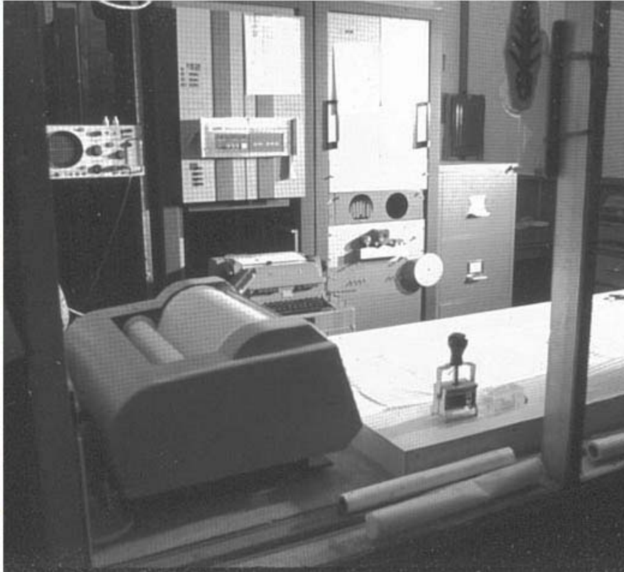
Packard-Bell PB250 computer with mercury delay-line memory.
