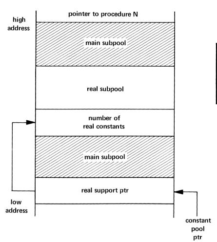
Figure 2-2 illustrates a constant pool with an embedded real subpool.
