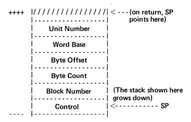
Figure 3-5. Stack State on Entering UNITREAD or UNITWRITE
