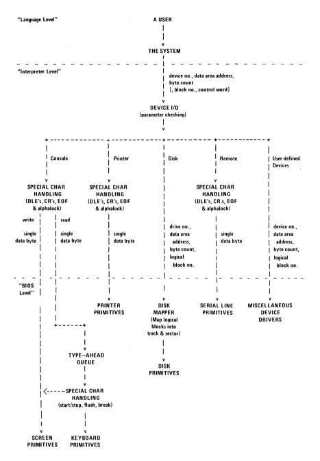
Figure 3-1. I/O Subsystem Hierarchy
