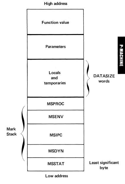
Figure 2-5. Procedure Activation Record
