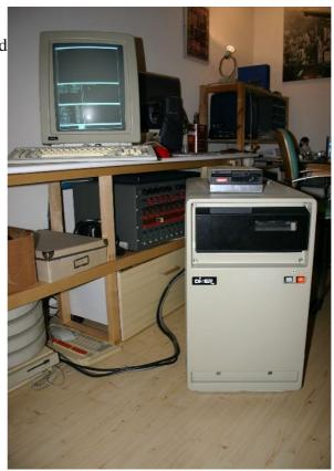
The Lilith has a 2901 bit-slice based architecture, uses a 128Kx16 main memory, a 704x928 monochrome high resolution display and a 10MB cartridge disk. The main memory can also be read in 64 bit chunks, as is done by the high resolution display and the Mcode instruction/data fetch unit.
