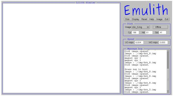
Note: the above picture shows a Lilith with the virtual disk in the offline state. It is not possible to boot in this state, the user needs to set the disk online.
