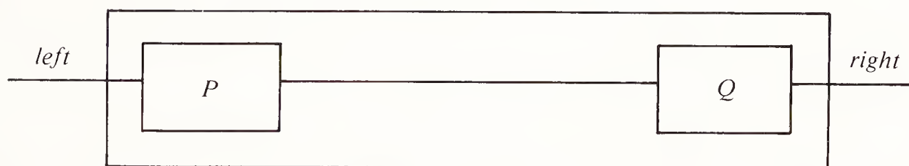
(d) The process (\text{chan } b \text{ in } C) with alphabet \{left, right\} .
